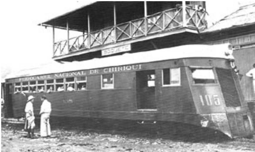
> Panama's Ferrocarril Nacional de Chiriquí operated an extensive fleet of Edwards Railcars. The image shows Chiriquí No. 105 at Boquete. This car was a streamlined version of the reliable Model 10 built in 1936. It was powered by a Buda engine and seated 30 passengers. Courtesy Cary Poole.
